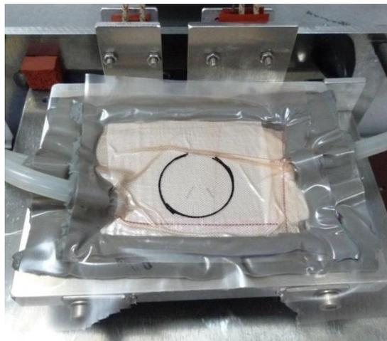
**Figure 1:** *Small heated vibrated mould with double vacuum bag set-up.*
